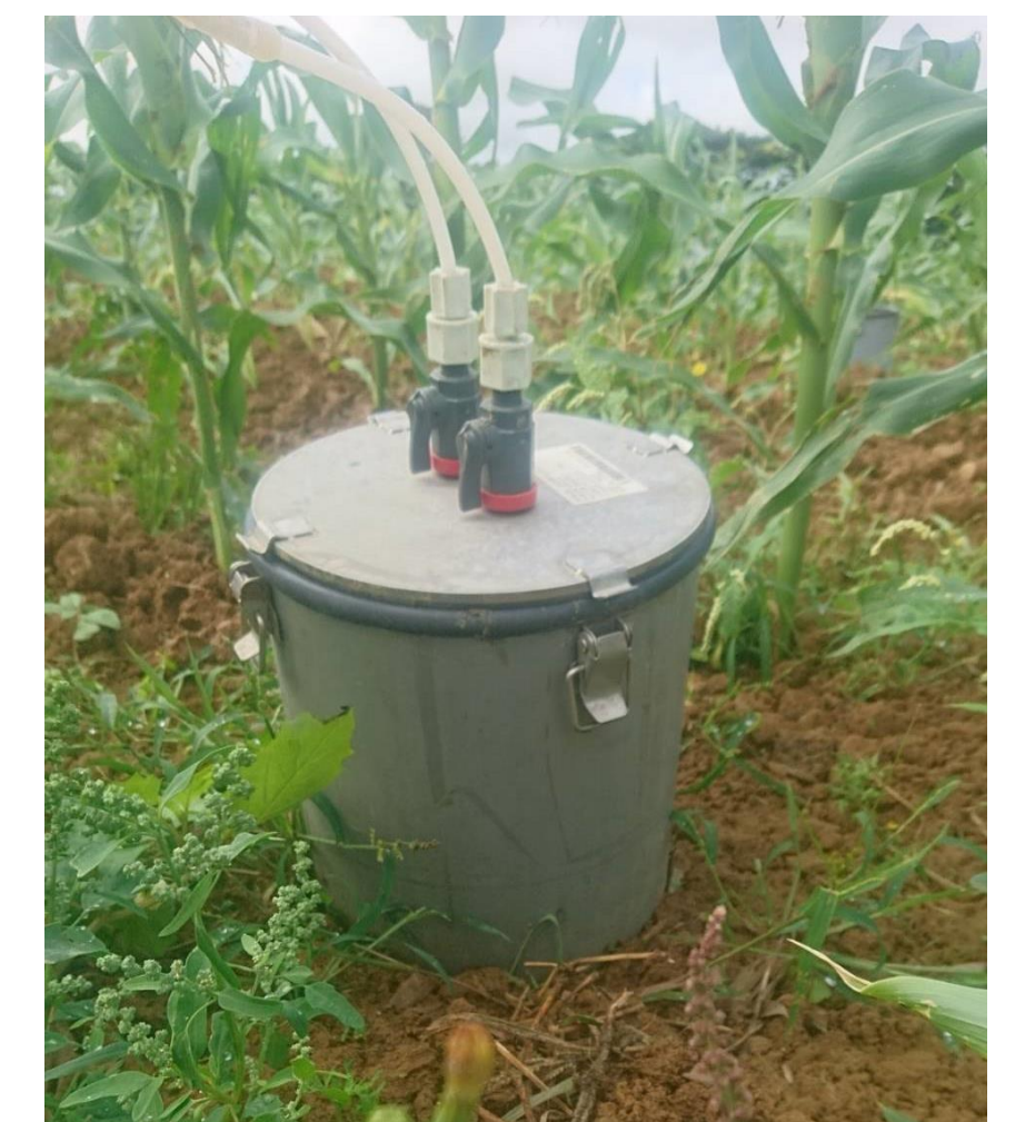
Fig.3 The GHG measured by closed chambers method.
